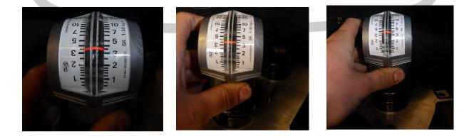
All readings need to be the same. If your throttles are out of balance, you should adjust the throttles with the higher readings. Adjustment can be made via the small bleed screws on
