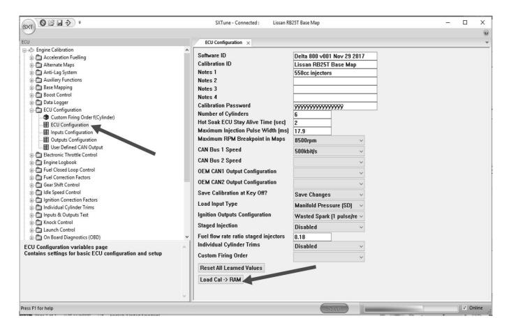
3. At the end of program loading you may see a message saying "programming failed SB". This is a temporary message at the Windows level and not related to the actual ECU programming, so this message can be ignored. Finally, click **save** at the bottom of the window. This will copy the cal from the SXTune software into the ECU. Disconnect and reconnect to the ECU and SXTune will load the new cal back from the ECU and into SXTune where you should be able to see the changes
