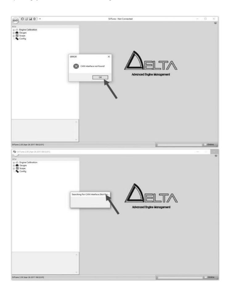
Additionally, it is possible for the existing firmware in the EUC to become corrupted, if for example a reliable ignition switch was not used for the switched supply or the cabling between the PC and the ECU was disturbed during programming. If this has happened the ECU will respond with the message below.
