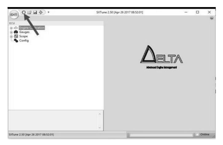
5. When SXT has connected successfully the green button will have a red circle with diagonal line as shown and the top information bar will say "Connected".
