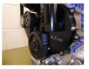
Install timing cover as per Standard part – ensure cam end float And timing is correct RS and RS+ 105 degs Full lift after tdc number 1 inlet at valve
