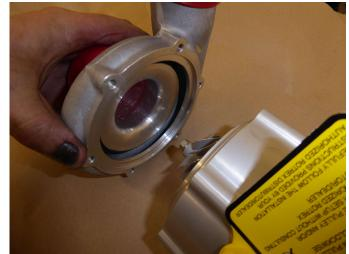
Undo these two bolts, carefully remove housing + turn 180 degress, tighten two silver bolts Attach charger to mounting bracket with long m5 bolts+blue Loctite – do not over tighten
