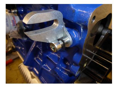
Alternator tensioner – use metric M8 and anti vibration washers Also note spacer location in Alternator and use long bolt Supplied through assembly
