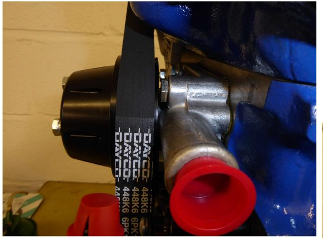
Install crank pulley as standard and belt run as shown Use alternator to tension belt
