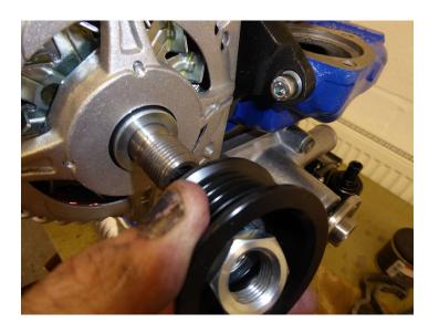
Remove old pulley and fit New supplied pulley
