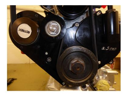
Idler pulley attach with blue Loctite and torque to 25 lb/ft Install as supplied orientation wise
