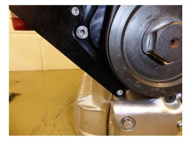
Supercharger bracket attaches with supplied unf <sup>1</sup>/<sub>4</sub> Fixings – use little blue Loctite and fully tighten
