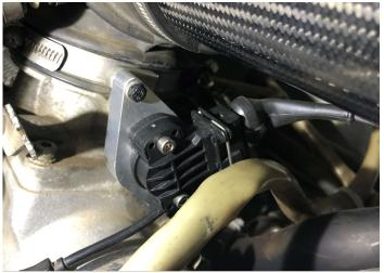
The supplied 5-way connector is for the inlet air temp sensor and new TPS. The 5-way male plug must be plugged into the 5 way female plug that came off the MAF sensor. See below picture.
