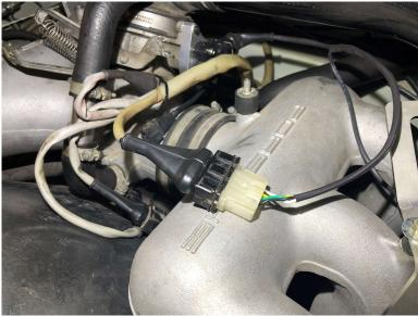
The new coil pack will use the original coils power supply. The coil wiring adapter has 2 ring terminals on that are different sizes. These need to be joined with the 2 different sized ring terminals from the standard coil as shown below. As a fail safe, the original coil wire colours should match the colours of the new adapter.
