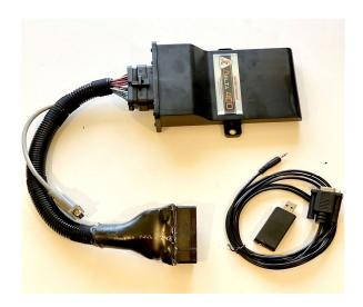
Fully 'plug and play' programmable ECU solution for single point injection (SPi) Minis.
