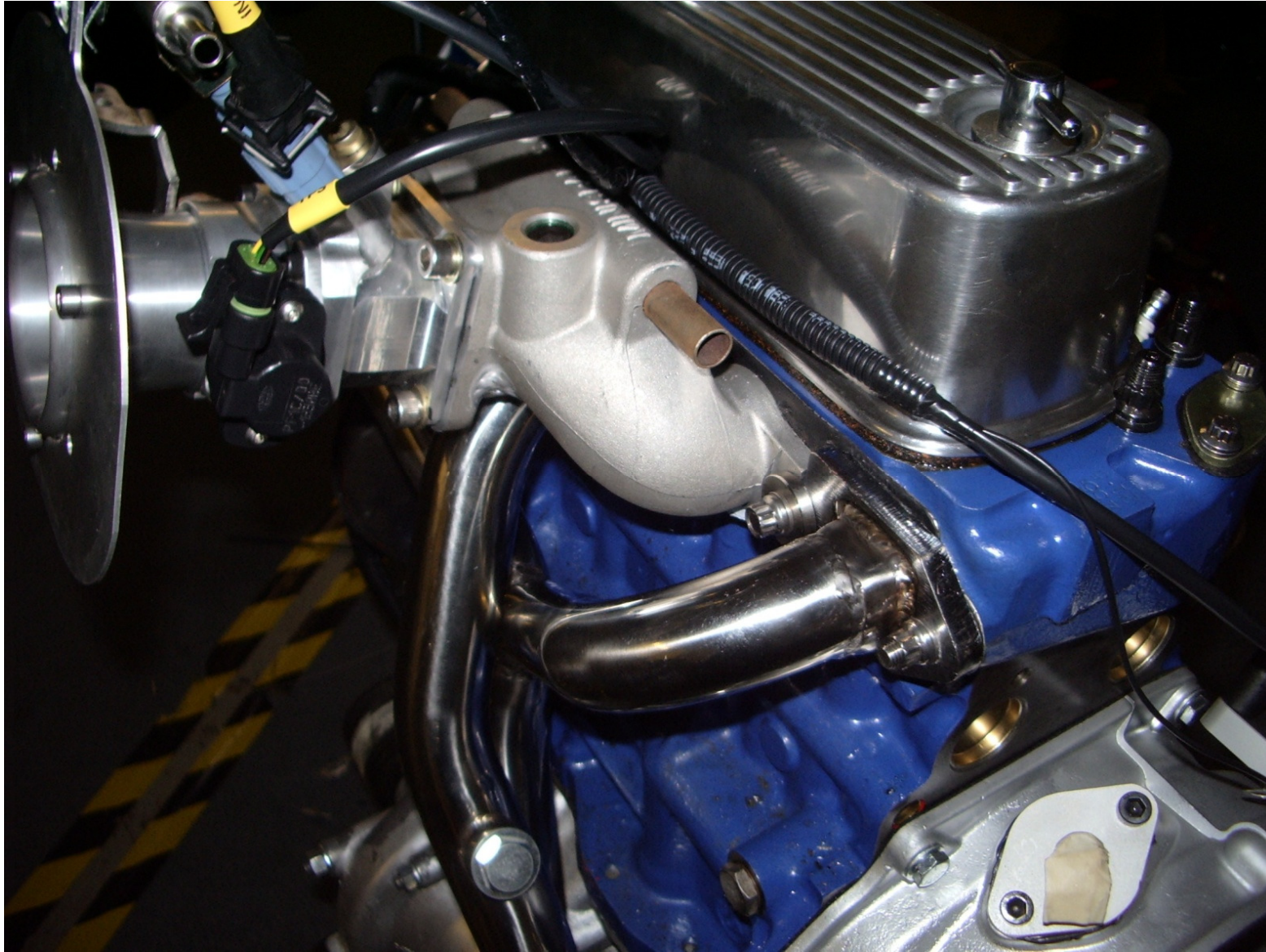
Basic cable routing around rear of cylinder head – clip wiring away from heat sources once installed
